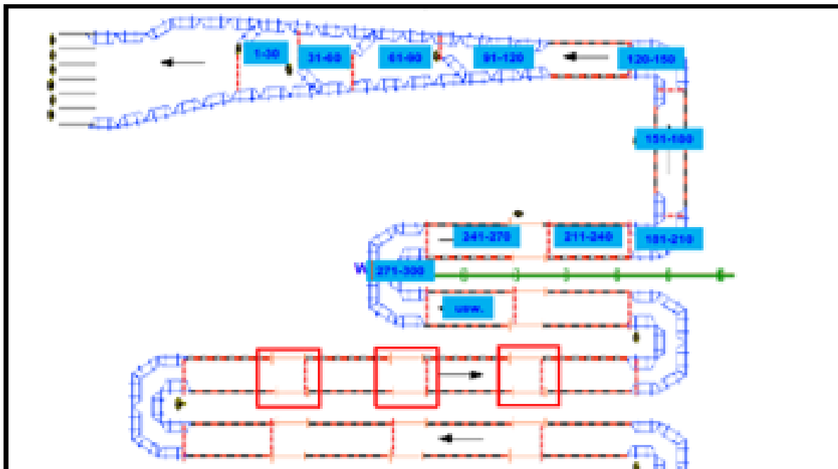
Figure 5: Example structure of a queuing system with infrastructural and organisational portioning by numbering (Source: Bernd Belka, Special Security Services Germany) [3].
